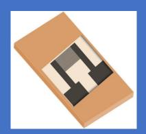
Thin film Ti/Pt based Inter Digitated Electrodes (IDEs) are fabricated on  $SiO_2/Si$ Substrate. IDEs with critical dimensions ranging from 2µm to 5µm (spacing between the IDE's being the same as width) are available. A combination of IDEs with microheater can also be provided for various tests like Gas sensing, testing for impedance, capacitance and conductivity measurements.
