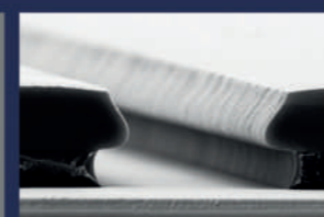
Bi-layer lift-off process
