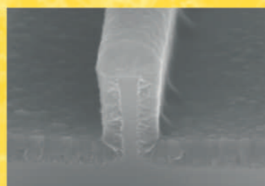
Conformal step coverage
