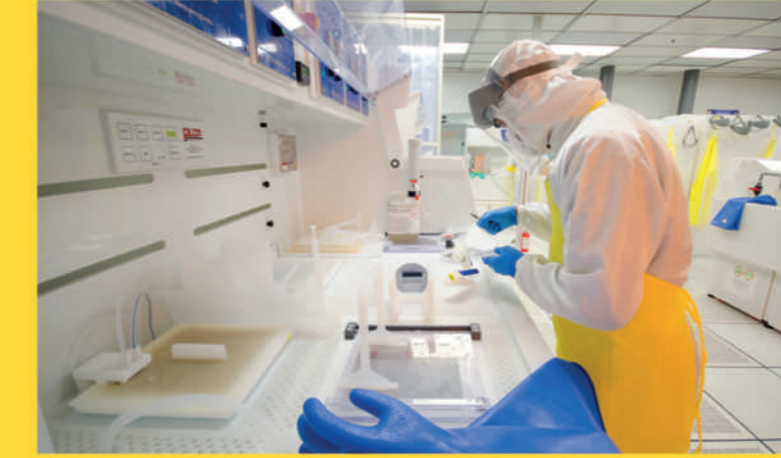
Dedicated wet benches to avoid cross-contamination
