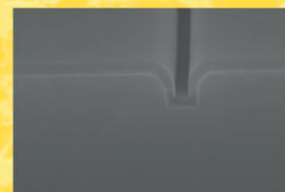
Conformal trench coverage
