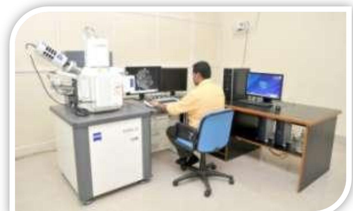
FE-SEM SUPRA 55 WITH AIR LOCK, EDS, EBSD
