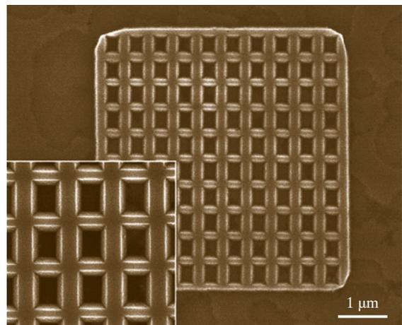
**Fig. 8.47** SEM image of an inverted truncated pyramid array fabricated on a silicon SOI wafer by SPM oxidation and subsequent etch in TMAH (pitch is  $500$  nm) (after [8.69])
