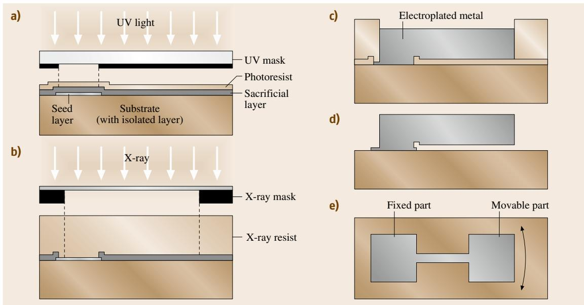
**Fig. 8.38a–e** Sacrificial LIGA process: (a) UV lithography for sacrificial layer patterning, (b) x-ray lithography, (c) electroplating, (d) structure releasing, and (e) top view of the movable structure
