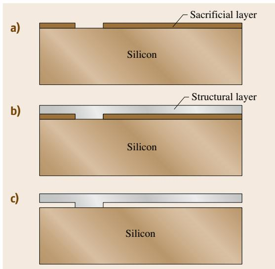
**Fig. 8.31a–c** Basic surface-micromachining fabrication process (a) silicon wafer with patterned sacrificial layer, (b) deposition and patterning of the structural layer, and (c) removal of the sacrificial layer
