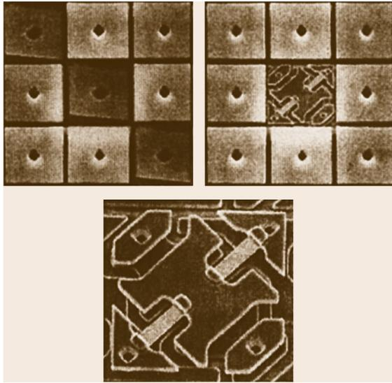
**Fig. 8.33** SEM images of the Texas Instrument micromirror array (after [8.30])
