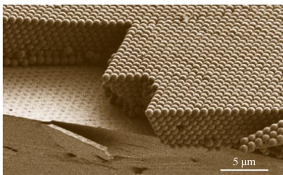
**Fig. 8.51** Cross-sectional SEM image of a thin planar opal silica template (spheres 855 nm in diameter) assembled directly on a Si wafer (after [8.91])
