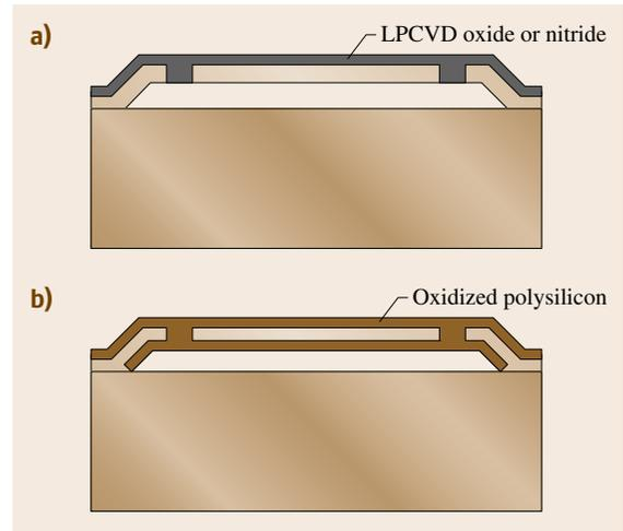
**Fig. 8.32a,b** Two sealing techniques for cavities created by surface micromachining
