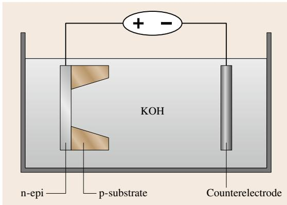
**Fig. 8.15** Electrochemical etch setup
