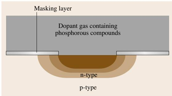
**Fig. 8.5** Formation of an n-type region on a p-type silicon substrate by diffusion of phosphorous
