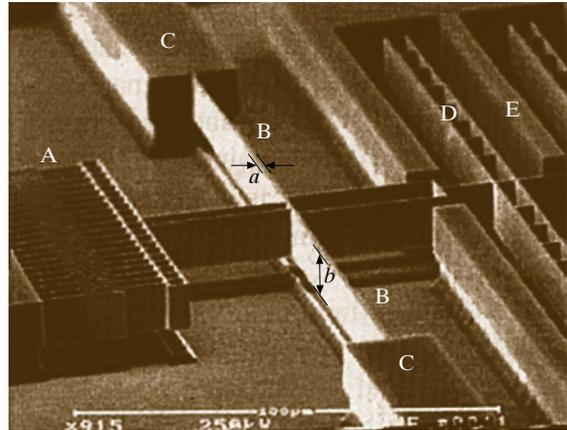
**Fig. 8.27** SEM image of a structure fabricated using the SCREAM process: A comb-drive actuator, B suspended spring, C spring support, D moving suspended capacitor plate, and E fixed capacitor plate (after [8.24])
