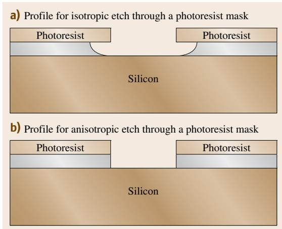
**Fig. 8.12a,b** Profile for (a) isotropic and (b) anisotropic etching through a photoresist mask
