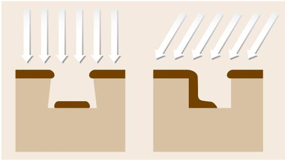
**Fig. 8.8** Shadow effects observed in evaporated films. Arrows show the trajectory of the material atoms being deposited
