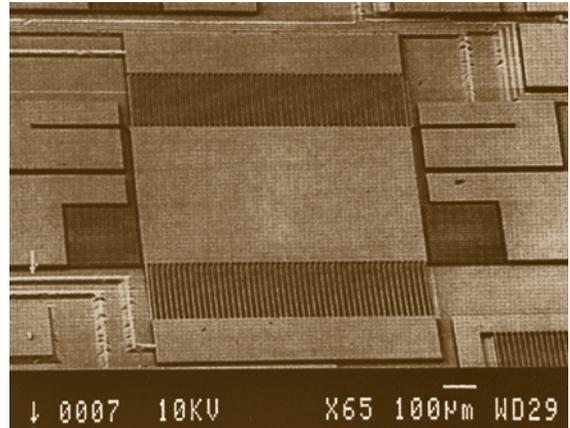
**Fig. 8.23** SEM image of a microaccelerometer fabricated using the dissolved wafer process (after [8.22])
