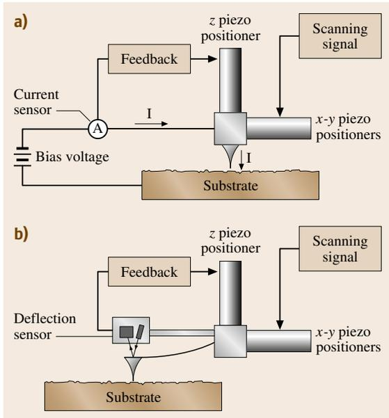
**Fig. 8.46a,b** Scanning probe systems: (a) STM and (b) AFM
