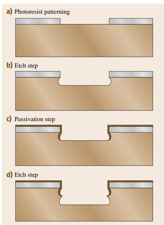
**Fig. 8.17a–d** DRIE cyclic process: (a) photoresist patterning, (b) etch step, (c) passivation step, and (d) etch step
