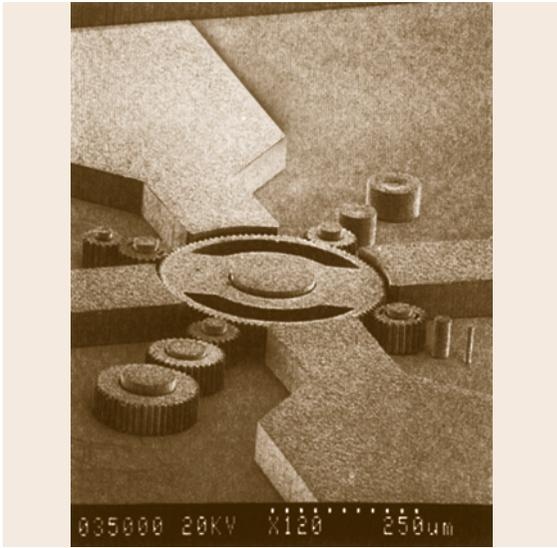
**Fig. 8.37** SEM of assembled LIGA-fabricated nickel structures (after [8.44])
