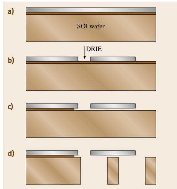
**Fig. 8.30a–d** DRIE processes using SOI wafers
