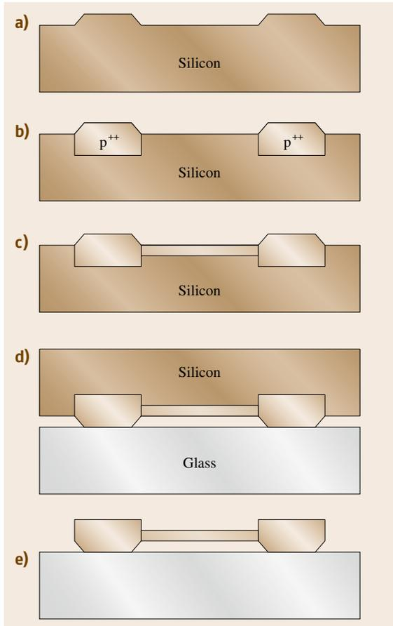
**Fig. 8.22a–e** Dissolved wafer process sequence: (a) KOH etch, (b) deep B diffusion, (c) shallow B diffusion, (d) silicon–glass anodic bond, and (e) release in EDP
