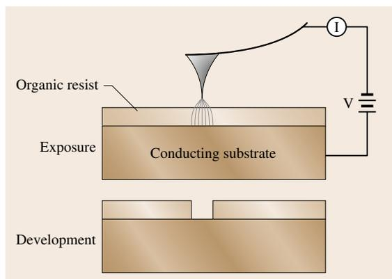
Fig. 8.48 Scanning probe lithography with organic resist
