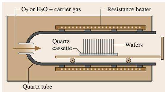
**Fig. 8.4** Schematic representation of a typical oxidation furnace
