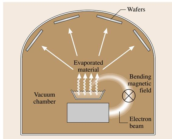
**Fig. 8.7** Schematic representation of an e-beam deposition system
