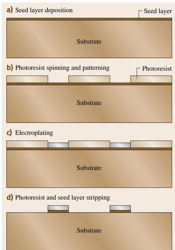
**Fig. 8.10a–d** Formation of isolated metal structures by electroplating through a mask: (a) seed layer deposition, (b) photoresist spinning and patterning, (c) electroplating, and (d) photoresist and seed layer stripping
