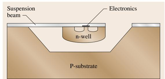
**Fig. 8.24** Suspended island created on a prefabricated CMOS chip using front-side wet etch and electrochemical etch stop
