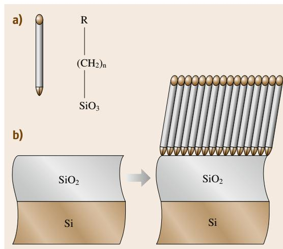
**Fig. 8.53** (a) Alkylsiloxane formed from the adsorption of alkyltrichlorosilane on Si/ $\text{SiO}_2$  substrates. (b) Schematic representation of the process
