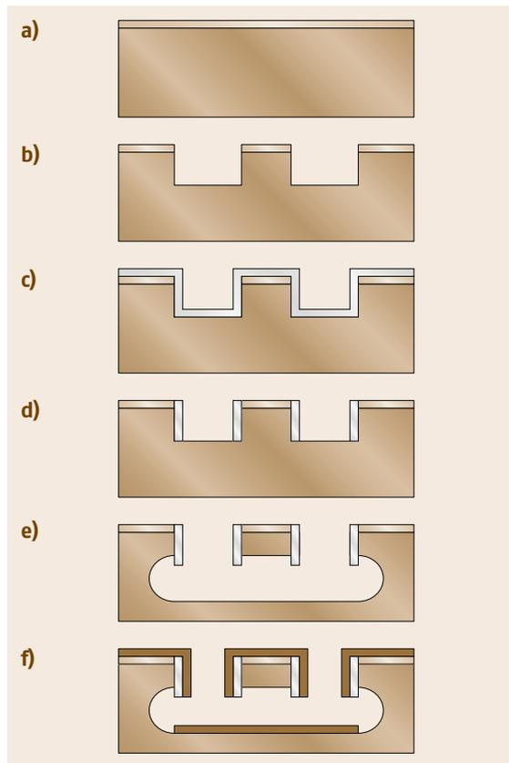
**Fig. 8.26a–f** Cross section of the SCREAM process (a) silicon wafer, (b) anisotropic silicon etch, (c) conformal passivation, (d) anisotropic etching of the passivation (hence protecting the sidewall), (e) isotropic silicon etch, and (f) metal deposition
