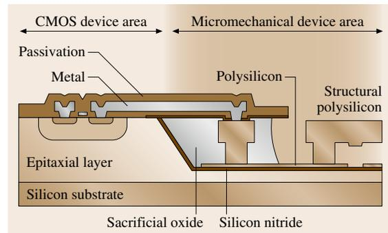
Fig. 8.35 Cross section of the Sandia MEMS-first integrated fabrication process
