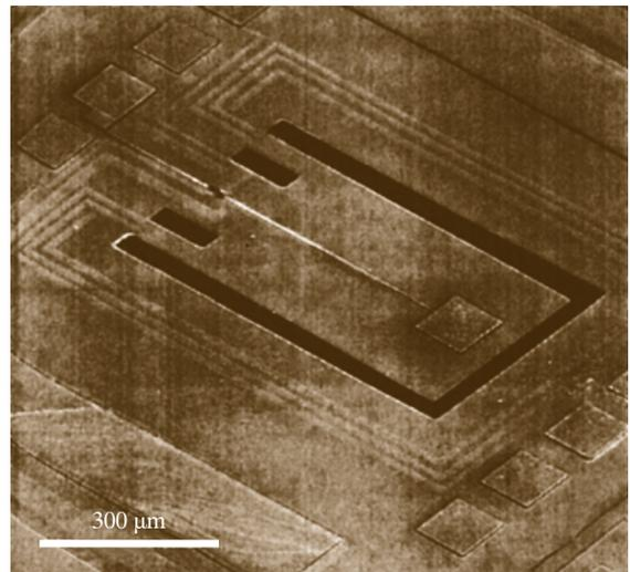
**Fig. 8.25** Photograph of a post-CMOS-processed cantilever beam resonator for chemical sensing (after [8.23])
