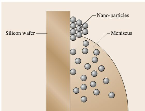
**Fig. 8.50** Colloidal particle self-assembly onto solid substrates upon drying in vertical position
