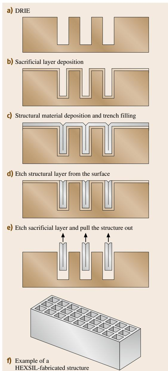
**Fig. 8.39a–f** HEXSIL process flow: (a) DRIE, (b) sacrificial layer deposition, (c) structural material deposition and trench filling, (d) etch structural layer from the surface, (e) etch sacrificial layer and pull the structure out, and (f) example of a HEXSIL-fabricated structure
