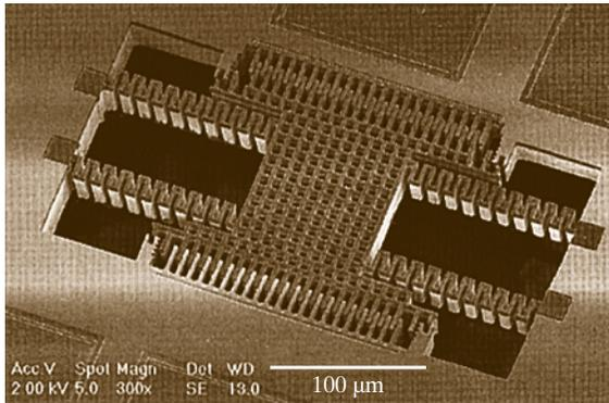
**Fig. 8.29** SEM image of a comb-drive actuator fabricated using aluminum-mask post-CMOS dry release (after [8.29])
