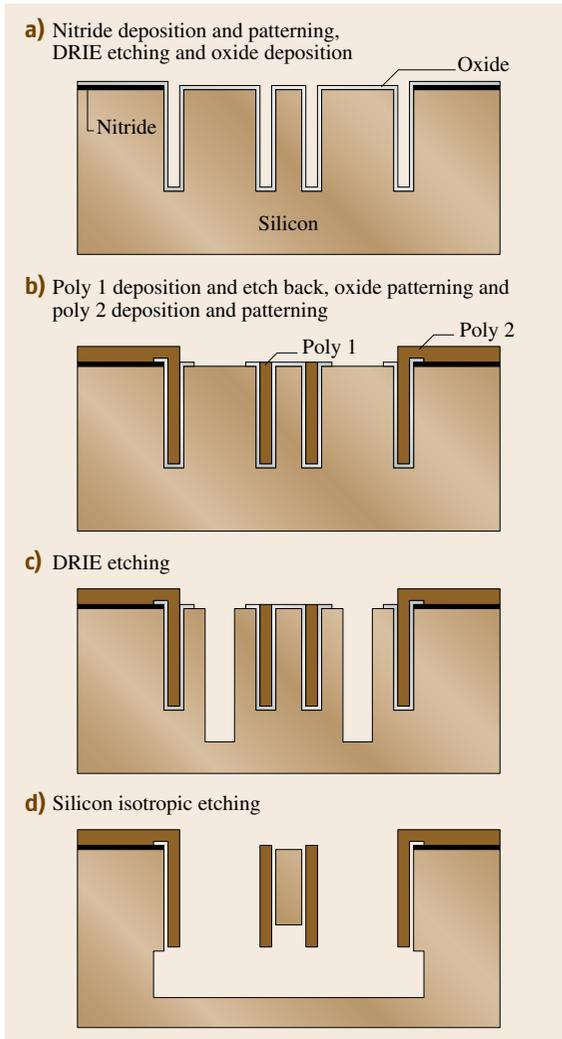
**Fig. 8.41a–d** HARPSS process flow: (a) nitride deposition and patterning, DRIE etching and oxide deposition, (b) poly 1 deposition and etch back, oxide patterning, and poly 2 deposition and patterning, (c) DRIE etching, and (d) silicon isotropic etching
