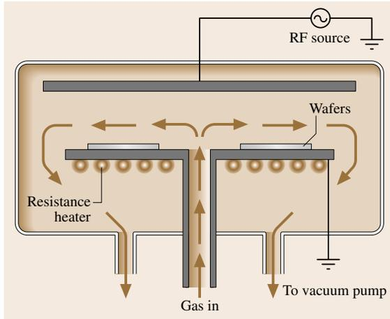
**Fig. 8.6** Schematic representation of a typical PECVD system
