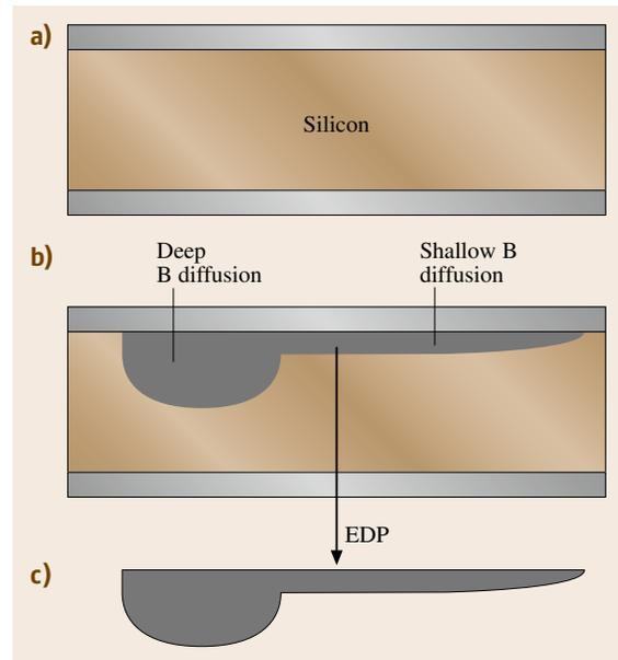
**Fig. 8.21a–c** Free-standing microstructure fabrication using deep and shallow boron diffusion and EDP release (a) silicon wafer, (b) deep and shallow boron diffusion, and (c) EDP etch
