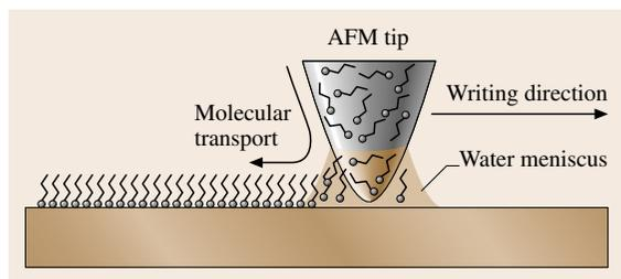
Fig. 8.49 Schematic representation of the working principle of dip-pen nanolithography
