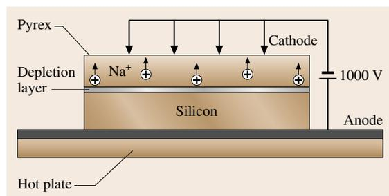
Fig. 8.18 Glass–silicon anodic bonding setup
