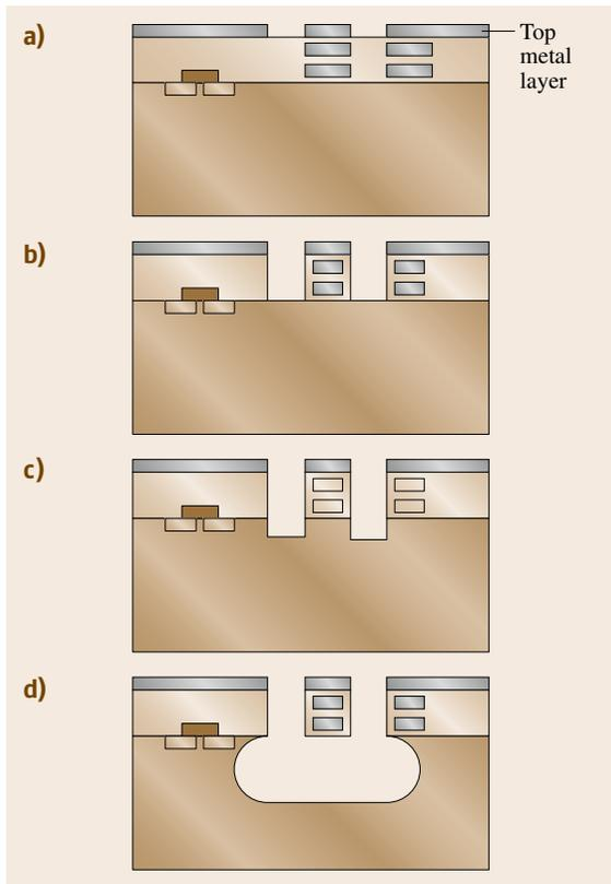
**Fig. 8.28a–d** Cross section of the process flow for post-CMOS dry microstructure fabrication
