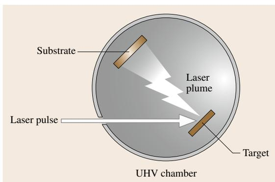
**Fig. 8.11** A typical PLD deposition setup
