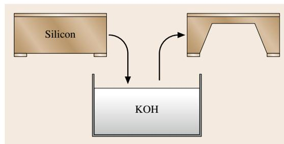
Fig. 8.19 Wet anisotropic silicon back-side etch
