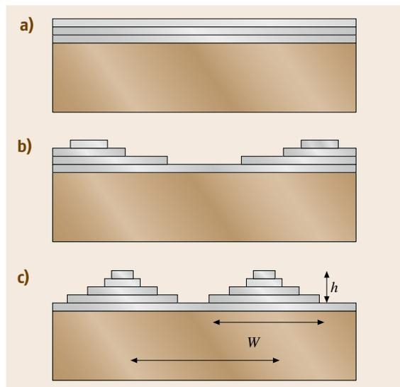
**Fig. 8.45a–c** Stranski–Krastanow growth mode, (a) 2-D wetting layer, (b) growth front roughening and breakup, and (c) coherent 3-D self-assembly
