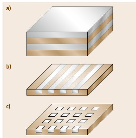
**Fig. 8.43a–c** Several important quantum confinement structures: (a) quantum well, (b) quantum wire, and (c) quantum dot
