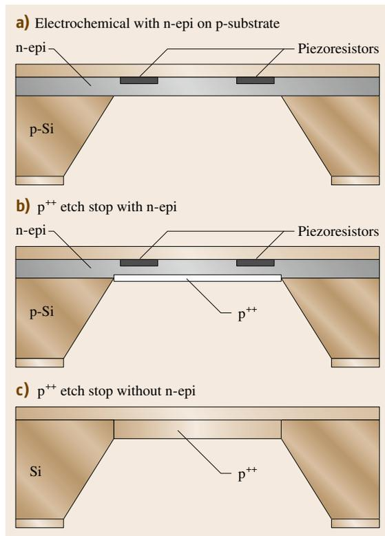
**Fig. 8.20a–c** Wet micromachining etch-stop techniques: (a) electrochemical with n-epi on p-substrate, (b)  $p^{++}$  etch stop with n-epi, and (c)  $p^{++}$  etch stop without n-epi
