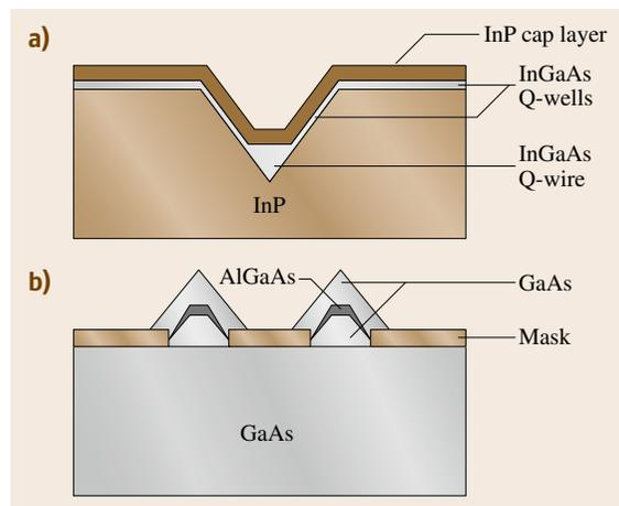
**Fig. 8.44** (a) InGaAs quantum wire fabricated in V-groove InP, and (b) AlGaAs quantum wire fabricated by epitaxial growth on a masked GaAs substrate
