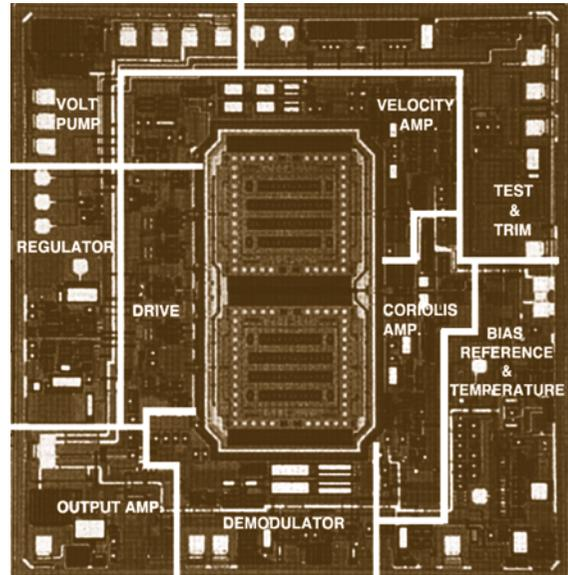
**Fig. 8.34** SEM image of the Analog Devices gyroscope (after [8.33])
