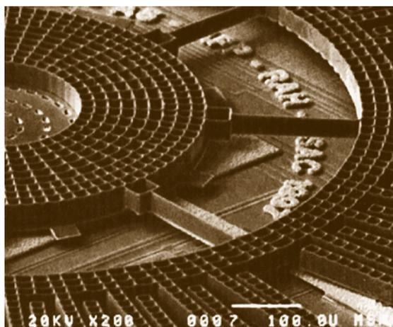
**Fig. 8.40** SEM micrograph of an angular microactuator fabricated using the HEXSIL process (after [8.47])
