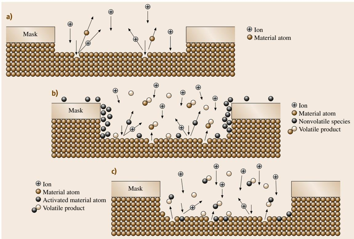
**Fig. 8.16a-c** Simplified representation of etching mechanisms for: (a) ion milling, (b) high-pressure plasma etching, and (c) RIE
