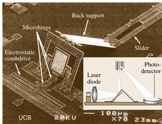
**Fig. 8.36** Silicon pin-and-sample hinge scanner with 3-D surface-micromachined structures (after [8.40])
