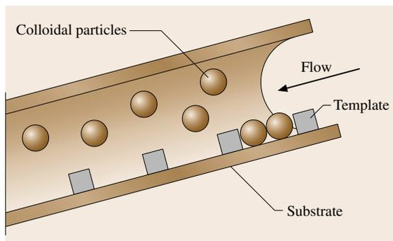
**Fig. 8.52** A cross-sectional view of the fluidic cell used for template-assisted self-assembly
